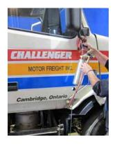
Test 1: In a test completed in May 2013 with Challenger Trucking on a Volvo truck, the DPF showed a soot level of 44%. After completing the service by using the ADI Exhaust Atomizer the soot level dropped to 18%. A regen was then run to complete the cleaning process and the final reading measured a soot level of only 2%. This represents a 96% reduction in the soot level of the DPF. The service time was approximately 1 hour.
